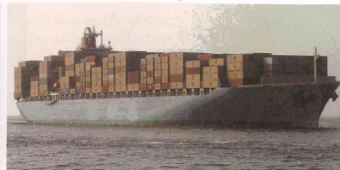
File picture of the 2006 built cellular container ship of Dwt. 72'968 MT, 6300 TEU capacity.
