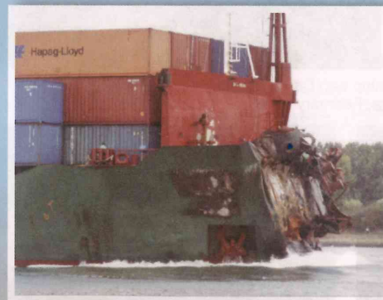
Vessel on her way back to port, the damage from the collision is clearly visible.
