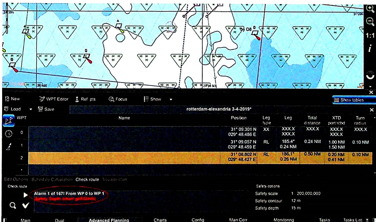
Figure 118: An inappropriately configured XTD can result in hundreds of alerts being generated. (Transas)
