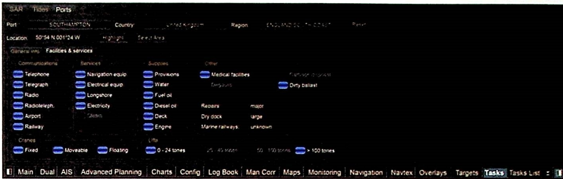
Figures 1 and 2: Some ECDIS manufacturers provide port databases that contain information such as restrictions, facilities and services. (Courtesy of Transas)
