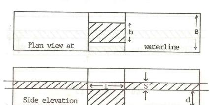
Note: Since the water-tight flat is far up, it will remain above the waterline after bilging. Its presence, therefore, makes no difference to the calculation.
