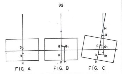
In the foregoing figures,  $GG_1$  is the transverse shift of COG. The couple formed by the forces of gravity and buoyancy causes the ship to incline. As the ship inclines, the COB shifts to the lower side, as explained in chapter 9, and when it comes vertically under  $G_1$ , the ship would be in static equilibrium. The angle of inclination at which this happens is the list —  $\theta$  in foregoing figure C.
