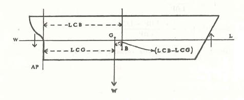
When the centre of buoyancy and the centre of gravity are not in the same vertical line, as shown in the figure, these two equal and opposite forces set up a couple tending to trim the vessel. The moment of this couple i.e. Trimming Moment, is obtained by the product of one of the forces and the lever between the forces i.e. (LCB - LCG)  $\times$  displacement. The Trimming Moment divided by the MCTC gives the trim in centimetres which is then divided by 100 to give the trim in metres.
