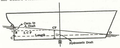
In the case illustrated above, the vessel is trimmed by the stern. Her hydrostatic draft is after draft – the correction AB. It can also be seen from the similar triangles ACD and ABF, that
