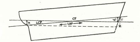
As shown in the above figure, the after trim would bear a ratio to the LCF as the total trim bears to the length of the ship, i.e.
