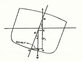
As can be seen from the figure, GZ = PN = KN - KP=  $KN - KG \sin \theta$
