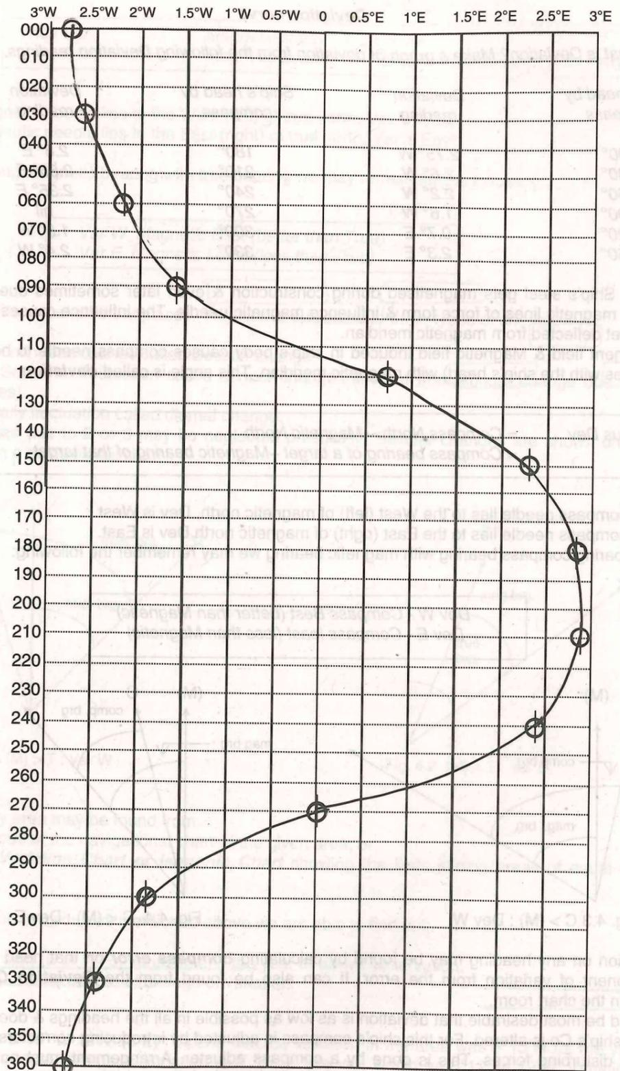
Fig. 4.5 Deviation graph as per the Deviation card.
