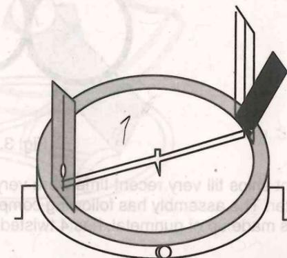
Note: Whenever gyro fails, power to the repeaters is switched off & the repeaters on each wing are adjusted to show 0 of card at lubber mark. Now repeaters can provide relative bearings. The repeaters in a way are being used as "fixed location pelorus".
