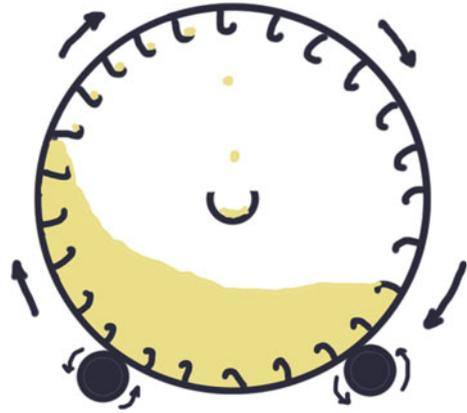
barrel until it reaches the top. It then falls from the scoop and lands in a tube that runs out of the barrel. In this way, the barley is cleaned so that only corns remain.
