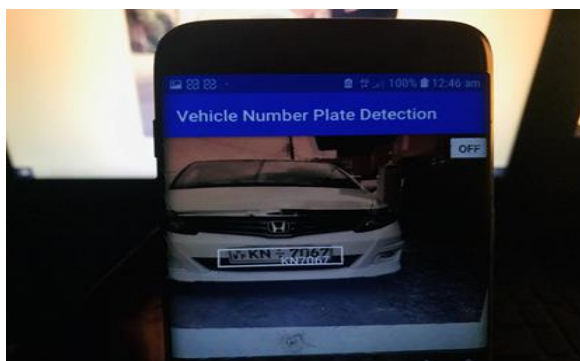
Figure 4: Number plate detection camera screen with flash light & zoom feature
