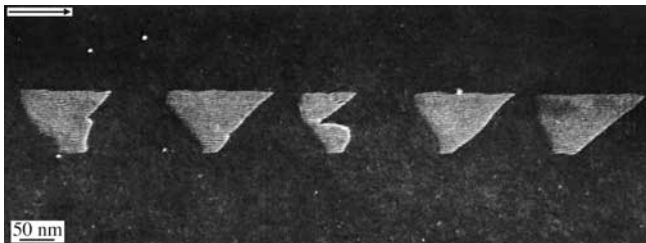
FIGURE 27.23. WB image showing the dissociation of a group of dislocations which are inclined to the foil surface and give wedge-shaped SFs. The shape of the SFs is caused by surface stresses.
