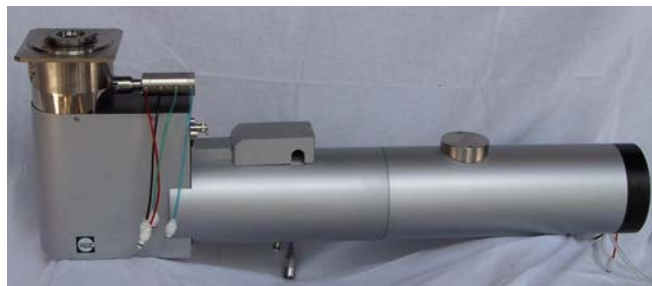
FIGURE 37.3. A Gatan Tridiem PEELS which interfaces below the viewing screen of an AEM.
