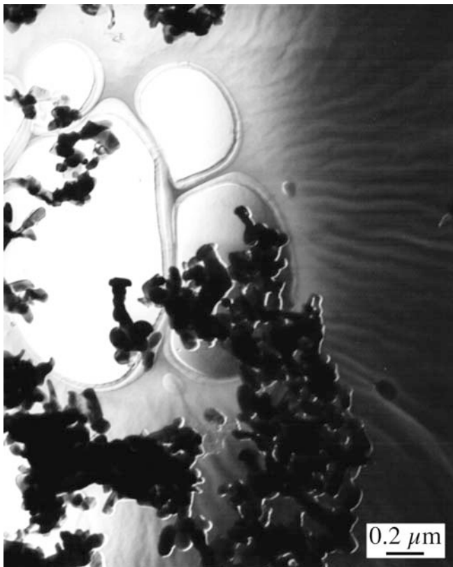
FIGURE 29.11. Topographic contrast from \text{Fe}_3\text{O}_4 particles on a carbon film. Ripples in the film are clearly visible. The shadow of the displaced objective diaphragm crosses the field of view.
