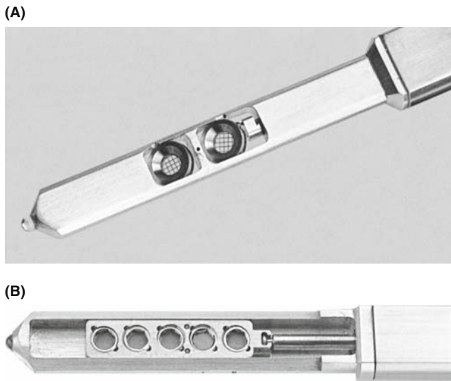
FIGURE 8.9. Multiple-specimen holders: (A) two-specimen double-tilt and (B) five-specimen single-tilt.
