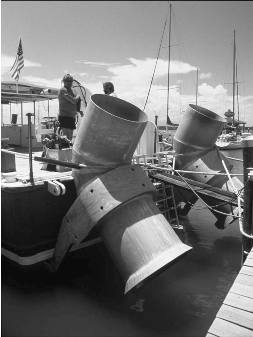
Fig. 16 The Florida treasure-hunting ship Rio Grande sporting enormous, tremendously destructive prop-wash deflectors on the stern (courtesy Donald H. Keith)
