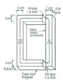
c) Hence, find required minimum current in a coil of 1000 turns wound on the cast iron to operate relay. (4 marks)
