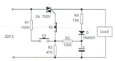
Power Failure Self-locking Switch
