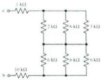
ii. Evaluate the equivalent resistance (RAB) of the following infinite network of resistance. (4 marks)
