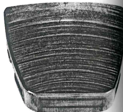
Figure 4.36 Effect of lubricant contamination. (Courtesy of Glacier Metal Company Ltd., Wembley, England.)
